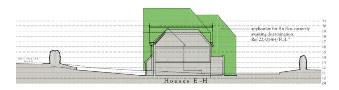
(Site section houses E- H showing differences between refused scheme for 6 flats at no.29 compared to the current application)
