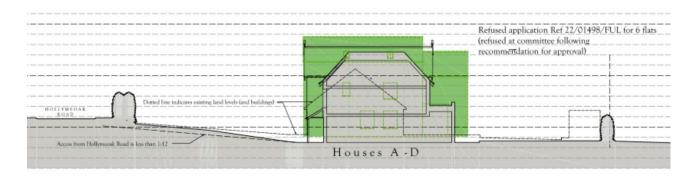
(Site section houses A – D showing differences between refused scheme for 6 flats at no.29 compared to current application)
